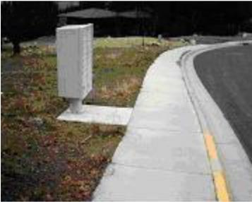
**CORRECT** - PLACING THE CBU BEHIND THE SIDEWALK INSTEAD OF NEXT TO THE STREET HELPS TO PROTECT THEM FROM VEHICLES WHILE NOT IMPEDING PEDESTRIANS OR WHEELCHAIRS.
