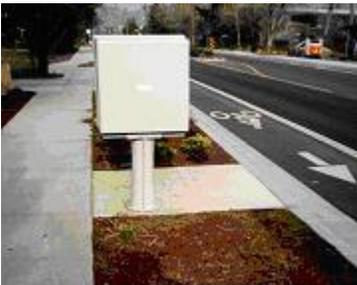
**CORRECT** - WHEELCHAIR ACCESSIBLE. SET BACK FROM THE ROADWAY. EASY ACCESS FOR THE CARRIER.
