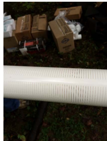
Slotted PVC pipe used for both air sparging in water and vapor extraction above the water level.
