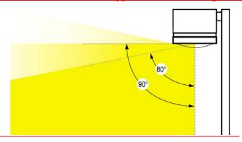
Shield is a device that is attached onto or inserted into a luminaire to alter the direction of light being emitted. A luminaire that has a shield attached or inserted is considered to be "shielded."
