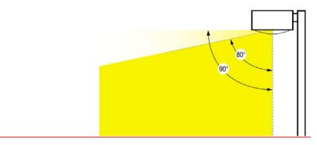
Full Cutoff means a luminaire light distribution where zero candela intensity occurs at or above an angle of 90° above nadir. Additionally the candela per 1,000 lamp lumens does not numerically exceed 100 (10 percent) at or above a vertical angle of 80° above nadir. This applies to all lateral angles around the luminaire.
