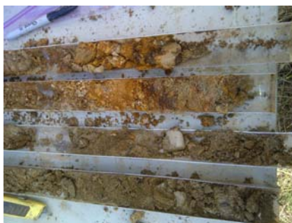
soil in a macro-core sample tubes from borehole MHP-01
