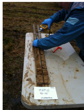
AMEC personnel using a PID to get measurements from soil collected between 50 and 55 feet below land surface at MHP-01
