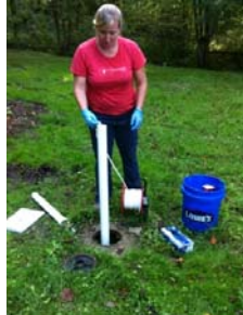
AMEC measuring water level in monitoring well MW-11A
