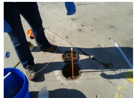
LNAPL being collected from PZ-2 for analysis
