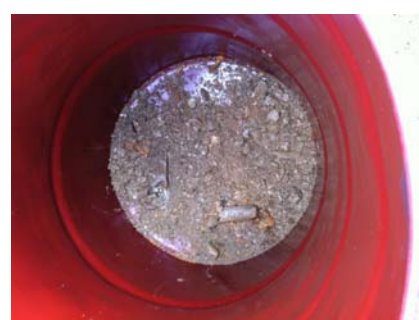
soil removed from boreholes placed in drums for future disposal
