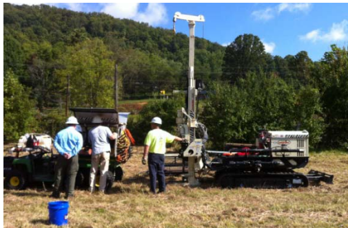
Data collection and boring at location MHP-01 The equipment on the right is the Geoprobe®. A gator utility vehicle (left) is used to carry the analyzers, computer, generator, etc.
