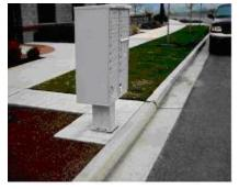
**INCORRECT –** LOCATED IN FRONT OF A PUBLIC OFFICE BUILDING - THE CBU SHOULD BE ACCESSIBLE FROM THE SIDEWALK.
