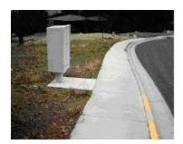
**CORRECT -** PLACING THE CBU BEHIND THE SIDEWALK INSTEAD OF NEXT TO THE STREET HELPS TO PROTECT THEM FROM VEHICLES WHILE NOT IMPEDING PEDESTRIANS OR WHEELCHAIRS.
